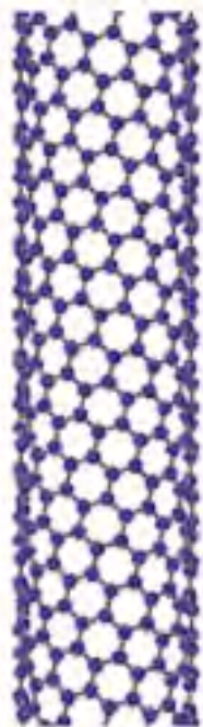
Figure 1b. Nanotube structure obtained by rolling a graphitic sheet into a cylinder.
